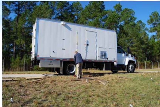
Leveling NRL Vehicle and marking effective Detector Center for Static Measurements
