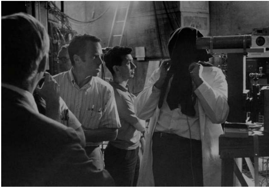
Figure 9. The first of a series of Apollo 13 eye flash experiments: Cornelius Tobias (under the black hood for dark-adaptation) positions his head in the neutron beam of the Rad Lab 184-inch cyclotron to observe eye flashes induced in the laboratory (Magnet, December 1970).
