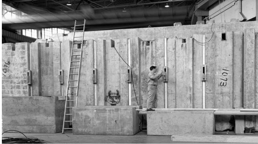
Figure 8. Concrete assembly for a 6 GeV proton shielding experiment at the Lawrence Radiation Laboratory. Michael Pick is seen inserting radiation detectors into the experiment. (1964)
