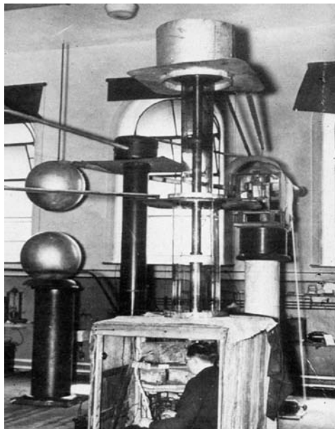
Figure 1. Photograph of the Cockcroft-Walton Accelerator. John Cockcroft is in the cabin observing nuclear disintegrations.
